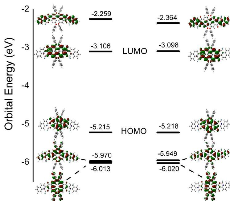
**Figure S13.** The frontier orbital energy levels and orbital maps of *cis* (left) and *trans* (right) isomer of **2**.
