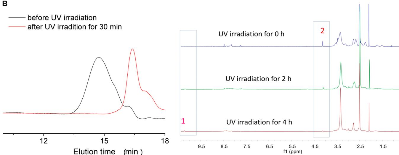
**Figure 3.** (A)  $^1\text{H}$  NMR spectra of the disulfide-containing poly(amidoamine) with 2-((2-nitrobenzyl)thio)ethanol terminals under UV irradiation. (B) GPC traces of disulfide-containing poly(amidoamine) with 2-((2-nitrobenzyl)thio)ethanol terminals before and after UV irradiation.
