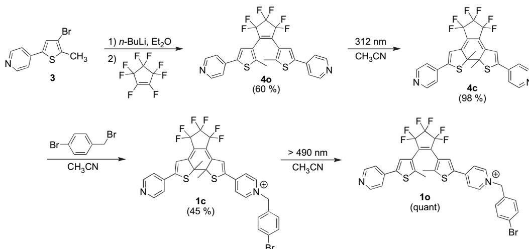
**Scheme 3.** Synthesis of ring-closed and ring-open isomers **1c** and **1o**. The counterions are  $\text{NO}_3^-$ .
