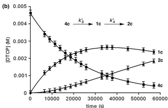
**Figure 4.** a) Changes in concentration of bis(pyridine) **4o** (□), monocation **1o** (○) and dication **2o** (△) when a CD<sub>3</sub>CN solution of **4o** ( $4.6 \times 10^{-3}$  M) is treated with excess 4-bromobenzyl bromide. (b) Changes in concentration of bis(pyridine) **4c** (■), monocation **1c** (●) and dication **2c** (▲) when a CD<sub>3</sub>CN solution of **4c** ( $4.6 \times 10^{-3}$  M) is treated with excess 4-bromobenzyl bromide.
