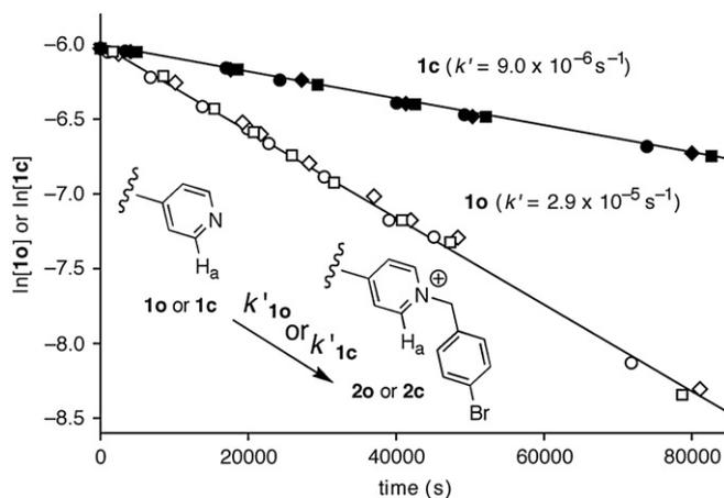
**Figure 2.** Changes in concentration of monocations **1o** (open symbols) and **1c** (filled symbols) when  $\text{CD}_3\text{CN}$  solutions of them ( $2.4 \times 10^{-3} \text{ M}$ ) are treated with excess 4-bromobenzyl bromide. The experiments were performed in triplicate.
