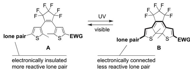
**Scheme 1.** The reversible photocyclization reaction of the dithienylcyclopentene backbone.
