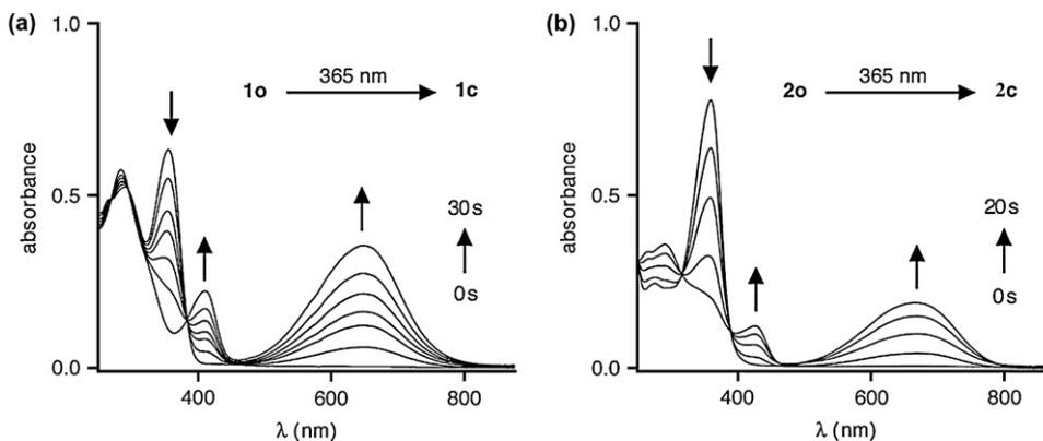
**Figure 1.** Changes in the UV–vis absorption spectra of  $\text{CH}_3\text{CN}$  solutions ( $2.0 \times 10^{-5} \text{ M}$ ) of (a) **1o** and (b) **2o** as they are irradiated with 365 nm light until the photostationary states are reached.
