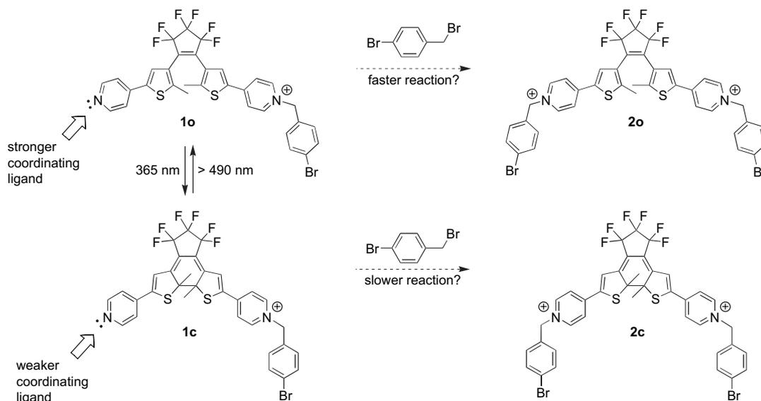
**Scheme 2.** Reversible photocyclization modulates the ability of the pyridine in **1o** and **1c** to act as a coordinating ligand. The alkylations of **1o** and **1c** to generate **2o** and **2c** are the model reactions described in this report.
