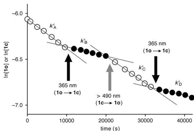
**Figure 3.** Modulation of the rate of the alkylation reaction of a CD<sub>3</sub>CN solution ( $2.4 \times 10^{-3}$  M) of DTCP **1** with excess 4-bromobenzyl bromide (30 mol equiv) by alternately irradiating with UV and visible light at 22 °C.<sup>24</sup>
