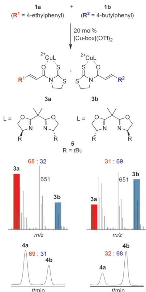
**Figure 1.** ESI-MS screening of the copper-catalyzed retro-DA reaction.
