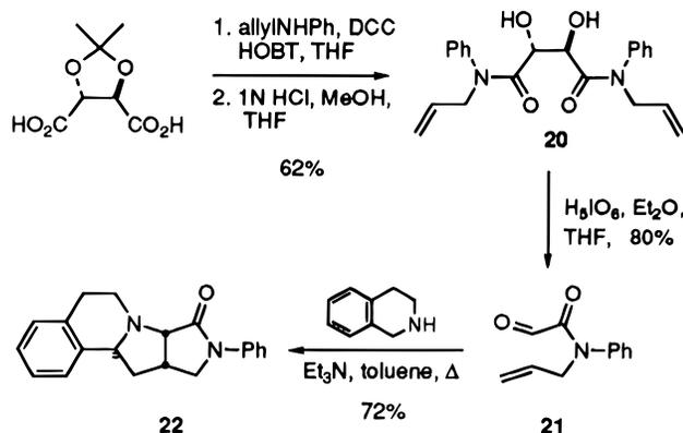
droisquinoline in refluxing toluene for 16 hours afforded the tetracyclic lactam **22** as a single diastereomer in 50% yield. Addition of one equivalent of triethylamine to the reaction mixture increased the yield to 72%; however, the yield was not affected when molecular sieves were added; these yields are based on the symmetrical tartramide and encompass the oxidation, condensation, and cyclization steps.
