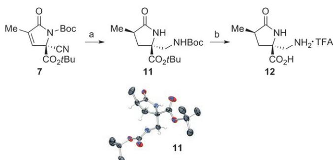
**Scheme 6.** Diastereoselective hydrogenation and amino acid synthesis. Reagents and conditions: a) 1. H<sub>2</sub> (10 bar), Pd/C, Boc<sub>2</sub>O, NEt<sub>3</sub>, EtOH/THF (5:3), RT, 16 h; 2. 20% Mg(ClO<sub>4</sub>)<sub>2</sub>, CH<sub>2</sub>Cl<sub>2</sub>, reflux, 22 h, 82% (over 2 steps); b) TFA/CH<sub>2</sub>Cl<sub>2</sub> (1:1), 3.5 h, RT, 86%. TFA = trifluoroacetic acid.
