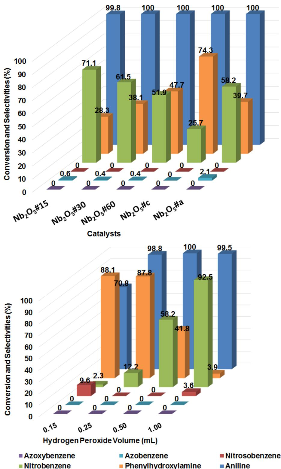
**Figure 4.** Aniline oxidation catalyzed by different Nb<sub>2</sub>O<sub>5</sub> catalysts (with 0.5 mL of H<sub>2</sub>O<sub>2</sub> and water as solvent) and effect of H<sub>2</sub>O<sub>2</sub> volume on oxidation of aniline over Nb<sub>2</sub>O<sub>5</sub>#60 catalyst (with acetonitrile as solvent).
