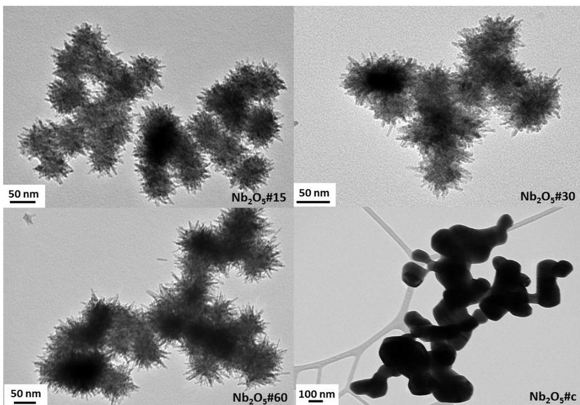
**Figure 2.** TEM images of Nb<sub>2</sub>O<sub>5</sub> catalysts.
