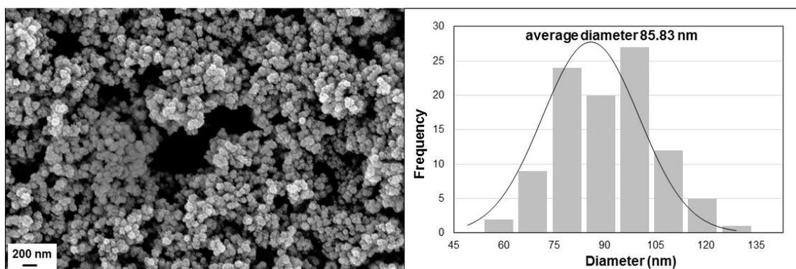
Figure 3. FE-SEM image and histogram of size distribution of Nb<sub>2</sub>O<sub>5</sub>#30 catalyst.
