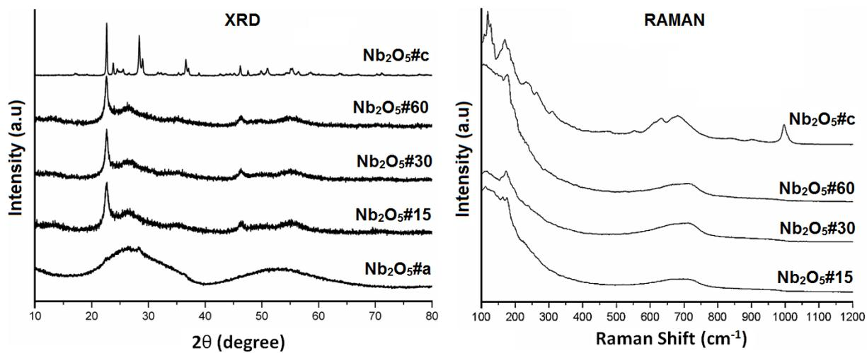
Figure 1. XRD patterns and Raman spectra of Nb<sub>2</sub>O<sub>5</sub> catalysts.
