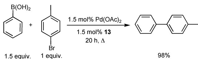
Scheme 6. Suzuki–Miyaura coupling reaction of phenylboronic acid with 4-bromotoluene utilizing Pd(OAc) 2 as catalyst and 13 as co-ligand.
