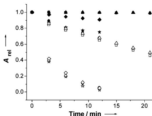
Figure 5. Changes in the Q-band absorbance of **4** (stars), **6** (circles), **7** (diamond), **8** (squares), and **12** (triangles) in water with 0.05% (w/v) Cremophor EL (all at 8.0  $\mu\text{M}$ ) with time, both in the absence (closed symbols) and presence (open symbols) of light ( $\lambda > 515$  nm, 118  $\text{mW cm}^{-2}$ ). The data were taken at 3 min intervals.
