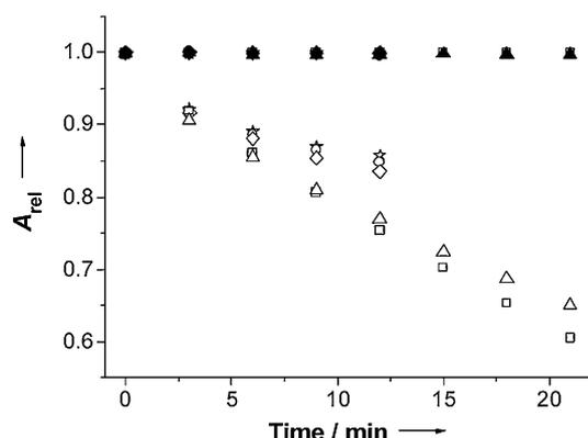
Figure 7. Changes in absorbance of RNO at 440 nm with time [initial [RNO] = 25.0  $\mu\text{M}$ ] using subphthalocyanines **4** (stars), **6** (circles), **7** (diamond), **8** (squares), and **12** (triangles) as the photosensitizers (all at 8  $\mu\text{M}$ ) in water with 0.05% (w/v) Cremophor EL, both in the absence (closed symbols) and presence (open symbols) of light ( $\lambda > 515$  nm, 118 mW  $\text{cm}^{-2}$ ). The data were taken at 3 min intervals ([imidazole] = 6.3 mM).
