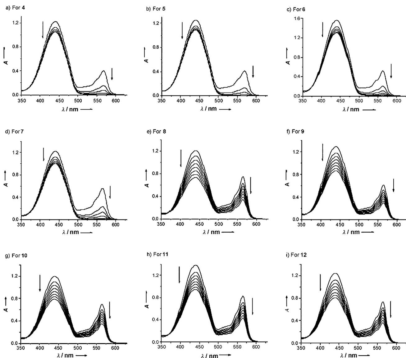
Figure 6. Changes in absorption spectra of mixtures containing **4–12** (8.0  $\mu\text{M}$ ), 0.05% (w/v) Cremophor EL, RNO (25.0  $\mu\text{M}$ ), and imidazole (6.3 mM) in water upon irradiation ( $\lambda > 515$  nm) with time. The spectra were taken at 3 min intervals. The relative rates of decay of RNO and the photosensitizer can be compared by monitoring the decrease in absorbance at 440 and 564–568 nm, respectively.
