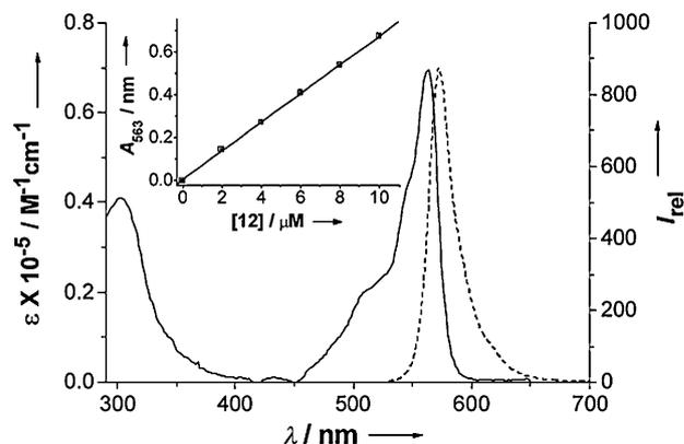
Figure 2. Electronic absorption (—) and fluorescence emission (---) spectra of **12** in DMF (2.0  $\mu\text{M}$ ). The inset plots the Q-band absorbance at 563 nm versus the concentration of **12**, showing that the Beer–Lambert Law is followed.
