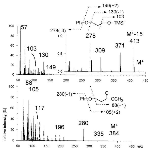
Figure 3. Mass spectra of metabolites with an alcohol and a carboxylic acid functional group at the C<sub>3</sub> side chain: 1-phytanyl-1-(propan-3-ol)ether (as TMSi-ether) and 1-phytanyl-1-(propanoic acid)ether (as methyl ester).
