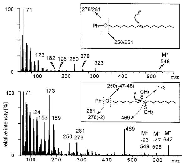
Figure 4. Mass spectra of the 1-phytanyl-1-octadec-9-enyl-ether with and without DMDS/J<sub>2</sub>-derivatization.
