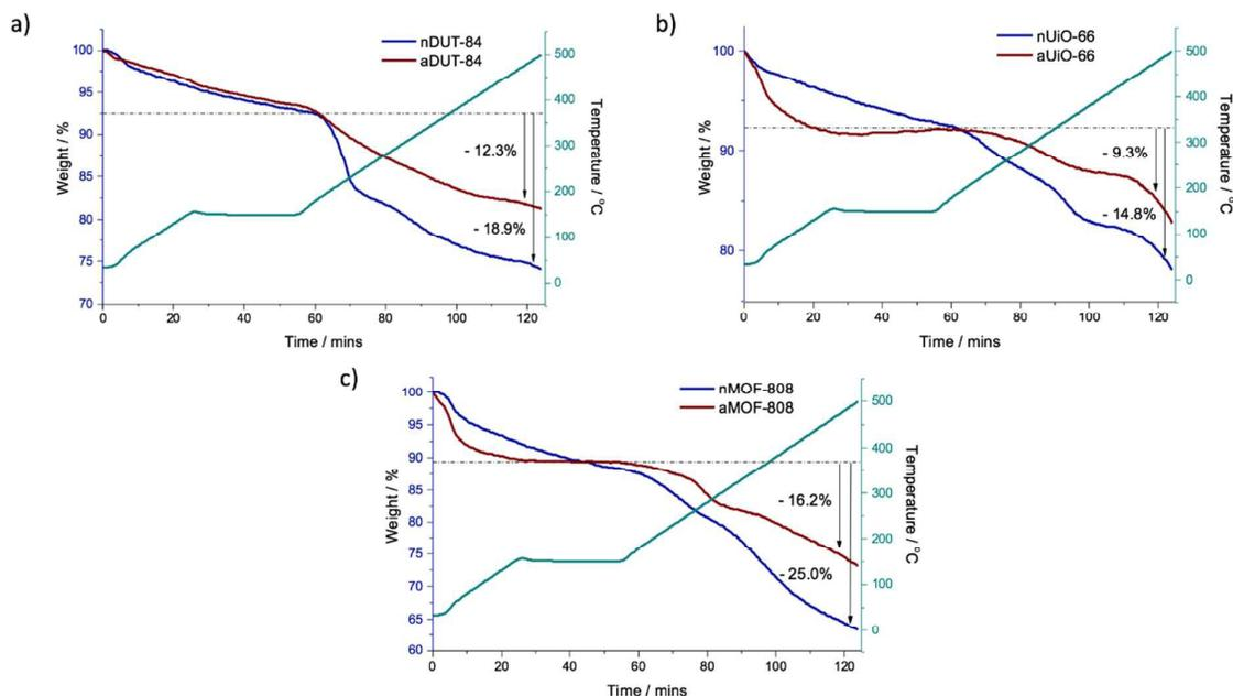
**Figure 3.** TGA trace for the non-activated and activated counterparts of each MOF. Heating rate:  $5\text{ }^{\circ}\text{C min}^{-1}$  in  $\text{N}_2$ , 30 min isotherm at  $150^{\circ}\text{C}$  followed by a ramp to  $500^{\circ}\text{C}$ . A value for the % weight loss post isotherm until end of the final ramp is shown on the TGA trace for each material.
