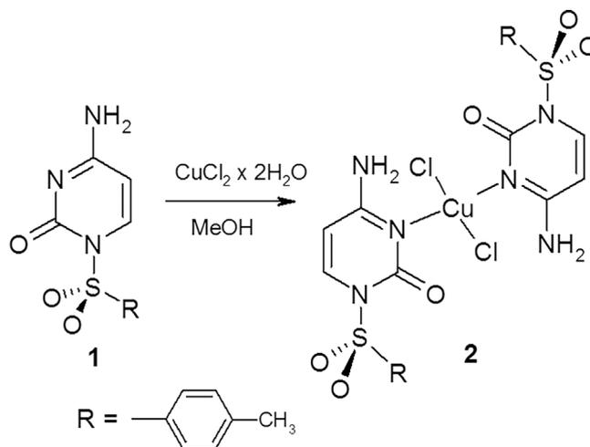
**Scheme 1.** Synthesis of Cu(1-TsC-N3)<sub>2</sub>Cl<sub>2</sub> (complex 2).
