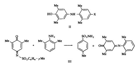
The peroxidase oxidation of 2,6-dimethylaniline therefore shows that the expected anil (I, X = H) was obtained, but not in high yield, indicating that additional substitution in the 4-position is necessary to prevent the formation of large quantities of ill-defined high molecular weight material. These results also show that 2,6-dimethylaniline is not a suitable donor for the quantitative determination of peroxidase activity.
