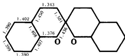
Fig. 9. Optimized geometry of SBP obtained by using the semi-empirical AM1 method (SCF level).
