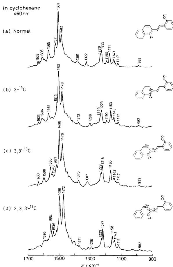
Fig. 7. Resonance Raman spectra of the transient species of <sup>13</sup>C substituted SBPs in cyclohexane taken 100 ns after UV (308 nm) irradiation: (a) normal species; (b) 2-<sup>13</sup>C species; (c) 3,3'-<sup>13</sup>C species; (d) 2,3,3'-<sup>13</sup>C species. Excitation wavelength, 460 nm; solvent bands have been subtracted.
