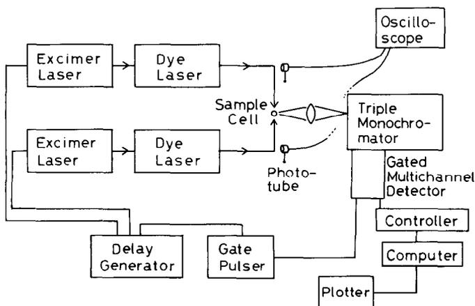
Fig. 2. Experimental system for time-resolved Raman spectroscopy.
