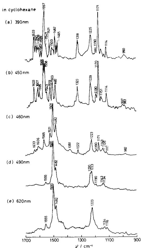
Fig. 6. Dependence of the resonance Raman spectra of the transient species of SBP in cyclohexane on the excitation wavelength: (a) 390 nm excitation; (b) 450 nm excitation; (c) 460 nm excitation; (d) 490 nm excitation; (e) 620 nm excitation. Spectra were measured at 100 ns after UV (308 nm) irradiation and the solvent bands have been subtracted.
