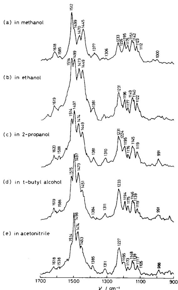
Fig. 4. Comparison of resonance Raman spectra of the transient species of SBP in various alcohols and in acetonitrile taken 100 ns after UV (308 nm) irradiation: (a) in methanol; (b) in ethanol; (c) in 2-propanol; (d) in *t*-butyl alcohol; (e) in acetonitrile. Concentration,  $2 \times 10^{-3}$  mol dm $^{-3}$ ; Raman excitation wavelength, 490 nm; solvent bands have been subtracted.
