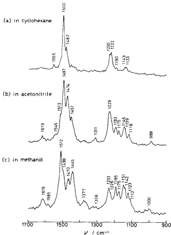
Fig. 3. Resonance Raman spectra of the transient species of SBP in different solvents taken 100 ns after UV (308 nm) irradiation: (a) in cyclohexane; (b) in acetonitrile; (c) in methanol. Concentration,  $2.0 \times 10^{-3}$  mol dm $^{-3}$ ; excitation wavelength, 490 nm; solvent bands have been subtracted.
