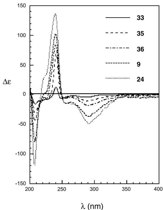
Figure 3. CD spectra of oligonaphthalenes in 0.4% dioxane–MeOH.
