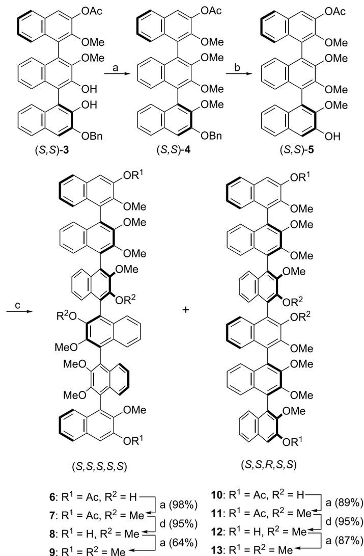
**Scheme 1.** The [3+3] construction of sexinaphthalenes. Reagents: (a) CH<sub>3</sub>I, K<sub>2</sub>CO<sub>3</sub>, 85%; (b) 10% Pd–C, H<sub>2</sub>, 97%; (c)  $\alpha$ -phenylethylamine, CuCl<sub>2</sub>, **6** (31%), **10** (38%); (d) K<sub>2</sub>CO<sub>3</sub>, MeOH.
