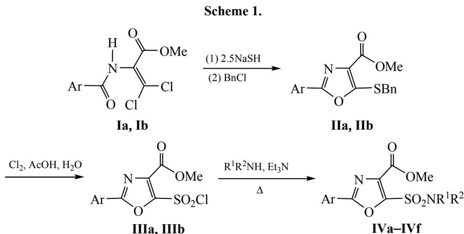
Ar = Ph (**I-IIIa**, **IVa-IVc**), 4-MeC<sub>6</sub>H<sub>4</sub> (**I-IIIb**, **IVd-IVf**); R<sup>1</sup>R<sup>2</sup>N = PhCH<sub>2</sub> (**IVa**, **IVd**), (CH<sub>2</sub>)<sub>5</sub>N (**IVb**, **IVe**), O(CH<sub>2</sub>)<sub>4</sub>N (**IVc**, **IVf**).
