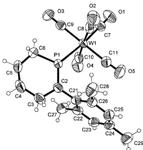
**Figure.** Structure of **17** in the crystal. Selected bond lengths [Å] and bond angles [°]: P1–C2 1.670(6), P1–C6 1.826(6), P1–W1 2.467(2), C2–C3 1.504(8), C3–C4 1.483(9), C4–C5 1.321(10), C5–C6 1.484(9), C2–C21 1.481(8); C2–P1–C6 107.9(3), C2–P1–W1 132.8(2), C6–P1–W1 119.3(2), P1–C6–C5 115.3(4), P1–C2–C3 124.2(4), P1–C2–C21 119.7(4), C3–C2–C21 116.2(5), C2–C3–C4 118.2(5), C3–C4–C5 126.2(6), C4–C5–C6 128.3(6).<sup>42</sup>
