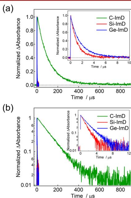
**Figure 4.** (a) Decay profiles of the transient biradicals of **C-ImD**, **Si-ImD**, and **Ge-ImD** ( $2.0 \times 10^{-4}$ ,  $2.0 \times 10^{-4}$ , and  $4.7 \times 10^{-4}$  M, respectively) in benzene at 298 K monitored at 570 nm upon 355 nm laser pulse irradiation (pulse width = 5 ns, power = 3.0 mJ/pulse). (b) The first-order plots for the decay profiles.
