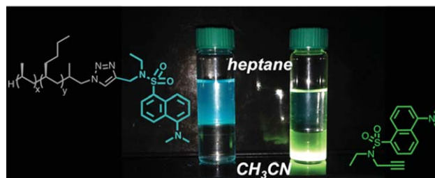
FIGURE 2 Photograph illustrating the phase-selective solubility of 6 (for heptane) compared to the selectivity of low molecular weight 5 (for acetonitrile) in a mixture of heptane and acetonitrile.
