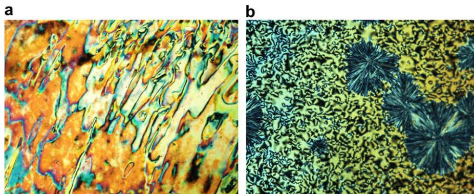
**Fig. 4.** Polarised optical micrograph of the nematic phase of **2b** at 60 °C (a) and of **6b** at 58 °C (b). In the later case the transition to the nematic phase occurs just before the crystallisation process.
