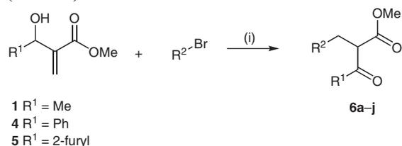
**Scheme 3** Reagents and conditions: (i) Pd(dbpf)Cl<sub>2</sub> (2.5 mol%), *N*-methyl-dicyclohexylamine (3 equiv), TBAC (20 mol%), DMF, 100 °C (closed tube).
