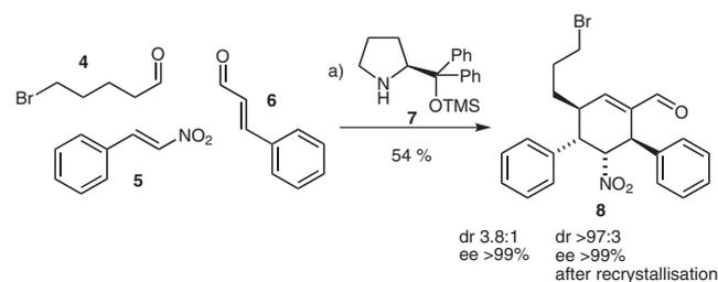
**Scheme 2** Triple domino reaction with 5-bromopentanal (**4**). *Reagents and conditions:* a) 0.2 M toluene, 20 mol% **7**, 24 h 0 °C, then 48 h, r.t.
