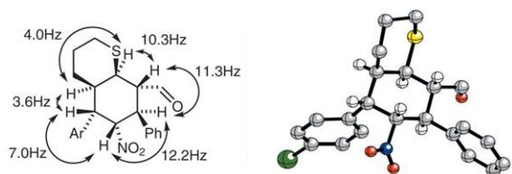
**Figure 1** Determination of the relative and absolute configuration of **14b** (Ar = 4- $\text{C}_6\text{H}_4$ ) by  $^1\text{H}$  NMR and X-ray analysis
