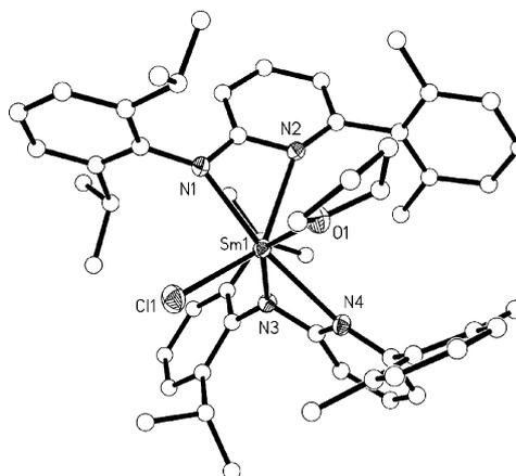
Figure 4. Molecular structure of **6**; selected bond lengths [Å] and angles [°]: N1–Sm1 2.334(2), N2–Sm1 2.572(2), N3–Sm1 2.352(2), N4–Sm1 2.519(2), O1–Sm1 2.4064(18), Cl1–Sm1 2.5681(6); N1–Sm1–N4 156.85(7), N1–Sm1–O1 103.58(7), N4–Sm1–O1 89.57(7), N1–Sm1–N3 107.83(7), N4–Sm1–N3 55.63(7), O1–Sm1–N3 144.80(7), N1–Sm1–N2 54.69(6), N4–Sm1–N2 107.57(6), O1–Sm1–N2 88.88(6), N3–Sm1–N2 96.43(7), N1–Sm1–Cl1 89.50(5), N4–Sm1–Cl1 109.53(5), O1–Sm1–Cl1 90.98(5), N3–Sm1–Cl1 104.61(5), N2–Sm1–Cl1 142.90(5).
