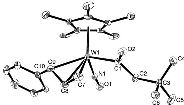
**Figure 5.** Solid-state molecular structure of **9** with 50% probability thermal ellipsoids. Selected interatomic distances (Å) and angles (deg): W(1)–C(1) = 2.240(5), W(1)–C(7) = 2.377(6), W(1)–C(8) = 2.345(5), W(1)–C(9) = 2.342(6), C(7)–C(8) = 1.409(8), C(8)–C(9) = 1.429(8), C(1)–O(2) = 1.222(6).
