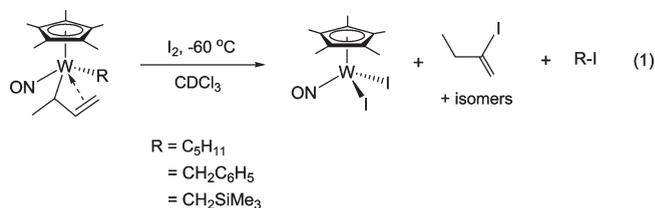
Compound **1** is also relatively stable toward oxygen and moisture in the crystalline state. However, reaction of **1** with aqueous hydrogen peroxide cleanly produces the known oxo peroxo complex Cp\*W(O)(η<sup>2</sup>-O<sub>2</sub>)(CH<sub>2</sub>SiMe<sub>3</sub>),<sup>8</sup> readily identifiable by its diagnostic <sup>1</sup>H NMR resonances. A plausible mechanism for the formation of the tungsten oxo peroxo complex is presented in Scheme 1.
