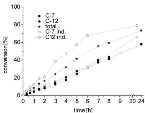
Figure 4. Conversion of acids and total conversion of both acids versus time for the competitive enzymatic esterification of combined heptanoic and dodecanoic acid with 3-phenylpropanol (filled symbols), all catalyzed by Lipase PS. Conversion rates from the initial slopes:  $C7_{ind}$ : 0.10;  $C12_{ind}$ : 0.21;  $C7$ : 0.08;  $C12$ : 0.07  $\text{min}^{-1}$ . The dotted lines are only a guide for the eye.
