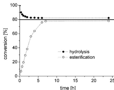
Figure 7. Hydrolysis and esterification of 3-phenylpropyl nonanoate catalyzed by Lipase PS versus time. The dotted lines are only a guide for the eye.
