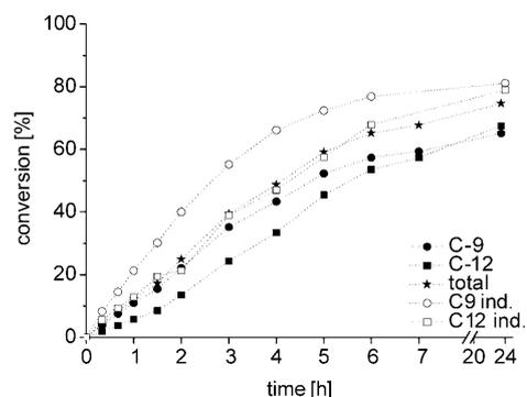
Figure 5. Conversion of acids and total conversion of both acids versus time for the competitive enzymatic esterification of combined nonanoic and dodecanoic acid with 3-phenylpropanol (filled symbols), all catalyzed by Lipase PS. Conversion rates from the initial slopes:  $C9_{ind}$ : 0.32;  $C12_{ind}$ : 0.21;  $C9$ : 0.19;  $C12$ : 0.11  $\text{min}^{-1}$ . The dotted lines are only a guide for the eye.
