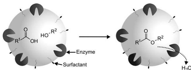
Figure 1. Schematic diagram of an esterification in the miniemulsion.
