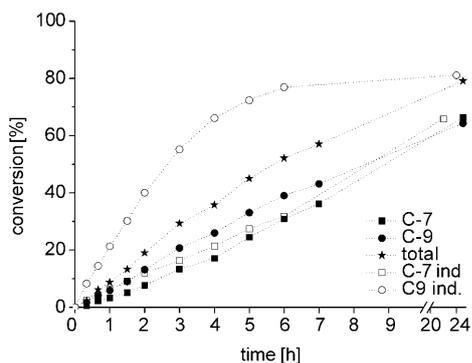
Figure 3. Conversion of acids and total conversion of both acids versus time for the competitive enzymatic esterification of heptanoic and nonanoic acid with 3-phenylpropanol (filled symbols), all catalyzed by Lipase PS. Conversion rates from the initial slopes:  $C7_{ind}$ : 0.10;  $C9_{ind}$ : 0.32;  $C7$ : 0.08;  $C9$ : 0.12  $\text{min}^{-1}$ . The dotted lines are only a guide for the eye.
