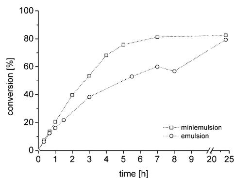
Figure 15. Reaction profiles of Lipase PS-catalyzed esterification of nonanoic acid with 3-phenylpropanol in macroemulsion relative to miniemulsion. The dotted lines are only a guide for the eye.
