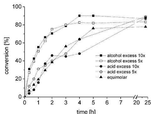
Figure 8. Reaction profiles of the Lipase PS-catalyzed esterification reactions of nonanoic acid with 3-phenylpropanol with an excess of alcohol (circles) or acid (squares) compared to the reaction with an equimolar amount of reactants. The reaction rates: the equimolar reaction: 0.32; excess of alcohol tenfold: 0.70; fivefold: 0.66; excess of acid tenfold: 0.22; fivefold: 0.25  $\text{min}^{-1}$ . The dotted lines are only a guide for the eye.
