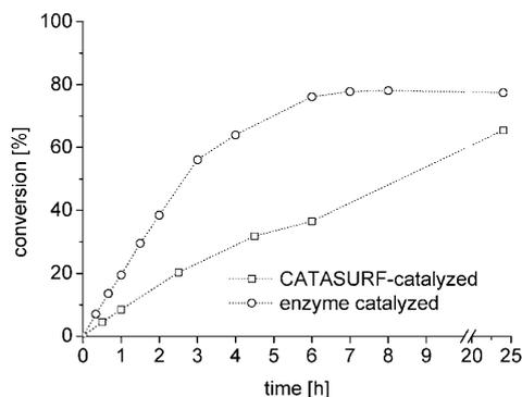
Figure 14. Comparison of conversion rates of DBSA and Lipase PS-catalyzed esterification of nonanoic acid with 3-phenylpropanol. Reaction rates: "CATASURF": 0.14; enzyme catalyzed: 0.32 min<sup>-1</sup>. The dotted lines are only a guide for the eye.
