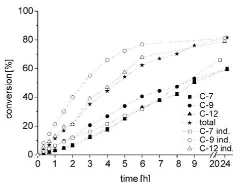
Figure 6. Conversion of acids and total conversion of all acids versus time for the competitive enzymatic esterification of combined heptanoic, nonanoic, and dodecanoic acid with 3-phenylpropanol (filled symbols), all catalyzed by Lipase PS. Conversion rates from the initial slopes:  $C7_{ind}$ : 0.10;  $C9_{ind}$ : 0.32;  $C12_{ind}$ : 0.21; C7: 0.06; C9: 0.11; C12: 0.06  $\text{min}^{-1}$ . The dotted lines are only a guide for the eye.
