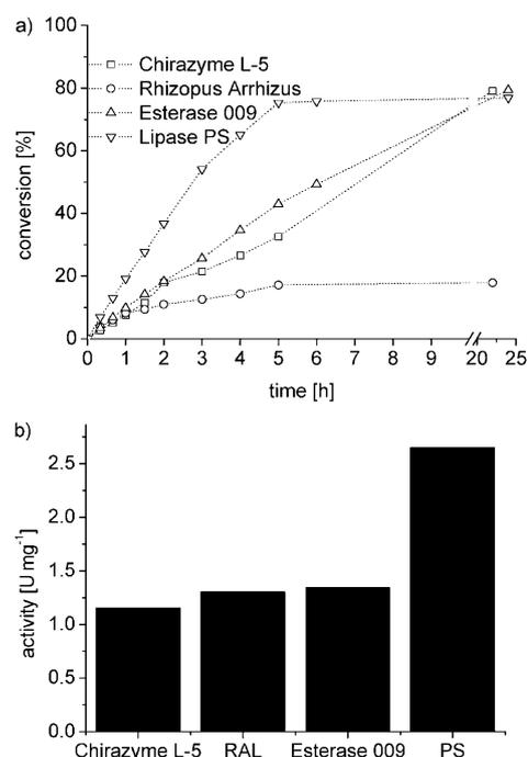
Figure 9. a) Enzyme-catalyzed reaction of nonanoic acid with 3-phenylpropanol with enzymes of different origins. The reaction rates: Chirazyme L-5:  $0.14$ ; *Rhizopus arrhizus* lipase:  $0.09$ ; Esterase 009:  $0.15$ ; Lipase PS:  $0.32 \text{ min}^{-1}$ . The dotted lines are only a guide for the eye. b) Calculated activities for the different enzymes in the esterification reaction of nonanoic acid with 3-phenylpropanol. RAL = *Rhizopus arrhizus* lipase.
