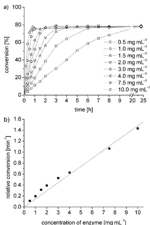
Figure 12. a) Reaction profile of the esterification of nonanoic acid with 3-phenylpropanol with different amounts of Lipase PS (0.5–10.0 mg mL<sup>-1</sup> with respect to the emulsion). The dotted lines are only a guide for the eye. b) Conversion per minute calculated from the initial slopes of the plot of conversion versus time. The dotted line is the linear fit of the data points.
