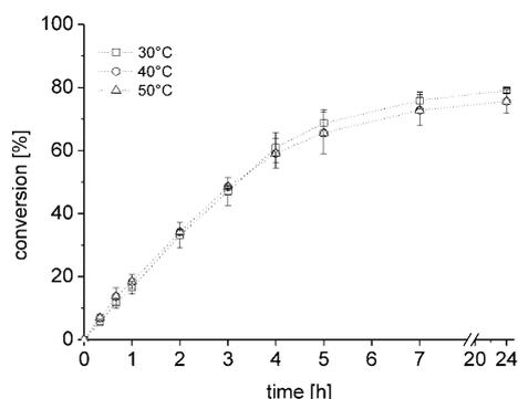
Figure 10. Influence of temperature on the reaction rate of the Lipase PS-catalyzed esterification of nonanoic acid with 3-phenylpropanol. The dotted lines are only a guide for the eye.
