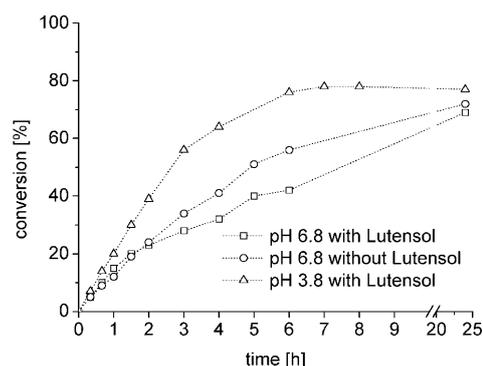
Figure 11. Reaction profiles of the Lipase PS-catalyzed esterification of nonanoic acid with 3-phenylpropanol in miniemulsions with continuous phases of pH 3.8 and 6.8, respectively. Conversion rates at pH 6.8: with Lutensol AT50: 0.16 min<sup>-1</sup>; without Lutensol AT50: 0.19 min<sup>-1</sup>; at pH 3.8: 0.32 min<sup>-1</sup>. The dotted lines are only a guide for the eye.
