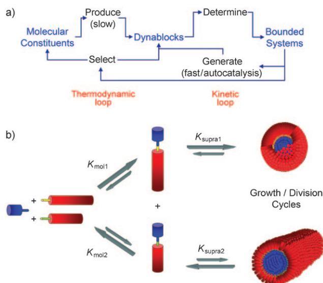
**Figure 4.** a) Synergistic constitutional relationships observed at two length scales within b) a model minimal self-replicating DCL. For clarity, the growth/division cycles of micellar structures are not represented.
