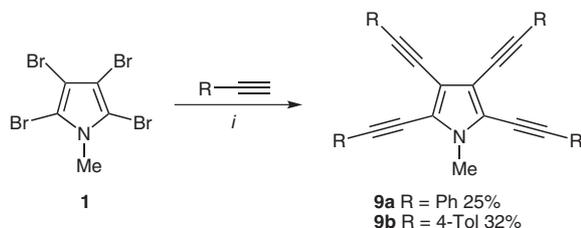
**Scheme 4** Synthesis of **9a,b**. Reagents and conditions: (i) **1** (1.0 equiv),  $\text{RC}\equiv\text{CH}$  (6.0 equiv),  $\text{PdCl}_2(\text{MeCN})_2$  (10 mol%),  $\text{CuI}$  (10 mol%),  $\text{Ph}_3\text{P}$  (20 mol%),  $i\text{-Pr}_2\text{NH}$ ,  $100^\circ\text{C}$ , 20 h.
