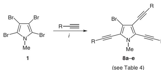
**Scheme 3** Synthesis of **8a–e**. *Reagents and conditions:* (i) **1** (1.0 equiv),  $\text{RC}\equiv\text{CH}$  (3.3 equiv),  $\text{PdCl}_2(\text{MeCN})_2$  (10 mol%),  $\text{CuI}$  (10 mol%),  $\text{Ph}_3\text{P}$  (20 mol%),  $i\text{-Pr}_2\text{NH}$ , 100 °C, 12–16 h.
