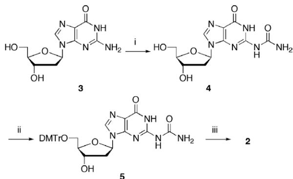
**Scheme 1.** Reagents and conditions: (i) a—TMSCl (5.0 equiv), pyridine, rt, 1 h; b—phenyl chloroformate (1.5 equiv), rt, 5 h; c—aqueous ammonia (10.0 equiv), pyridine, rt, 1 h, 55%; (ii) DMTrCl (1.5 equiv), pyridine (5.0 equiv), DMF, rt, 4 h, 84%; (iii) (CEO)P[N(*i*-Pr)<sub>2</sub>]<sub>2</sub> (1.3 equiv), 1*H*-tetrazole (0.6 equiv), (*i*-Pr)<sub>2</sub>NH (0.6 equiv), CH<sub>2</sub>Cl<sub>2</sub>, rt, 2 h, 90%.
