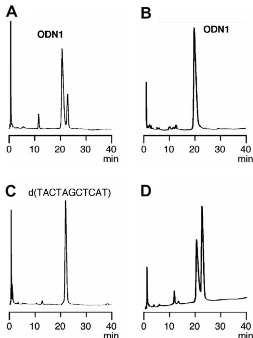
**Figure 2.** Anion-exchange HPLC analysis; 30 °C, 0.75 ml/min 20–22% B in 40 min. (A) Crude **ODN1** synthesized using **2**, (B) **ODN1** synthesized using 6-*O*-protected **1**, (C) 5'-d(TACTAGCTCAT)-3', and (D) mixture of **ODN1** synthesized from **2** and 5'-d(TACTAGCTCAT)-3'. The peak near 0 min is the injection peak.
