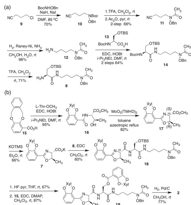
**Scheme 1.** (a) Synthesis of amine fragment **8**. (b) Completion of total synthesis of fimsbactin B (**2**).
