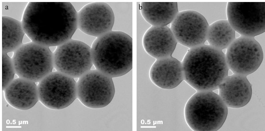
**Fig. 1.** TEM micrographs of (a)  $\text{Fe}_3\text{O}_4/\text{P}(\text{GMA-AA-MMA})$  and (b)  $\text{Fe}_3\text{O}_4/\text{P}(\text{GMA-AA-MMA})\text{-Pd}$ .
