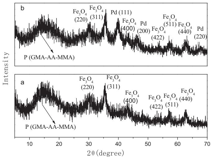
**Fig. 2.** XRD pattern of (a)  $\text{Fe}_3\text{O}_4/\text{P}(\text{GMA-AA-MMA})$  and (b)  $\text{Fe}_3\text{O}_4/\text{P}(\text{GMA-AA-MMA})\text{-Pd}$ .
