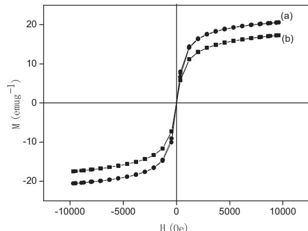
**Fig. 3.** The magnetization curve measured at room temperature for (a)  $\text{Fe}_3\text{O}_4/\text{P}(\text{GMA-AA-MMA})$  and (b)  $\text{Fe}_3\text{O}_4/\text{P}(\text{GMA-AA-MMA})\text{-Pd}$ .
