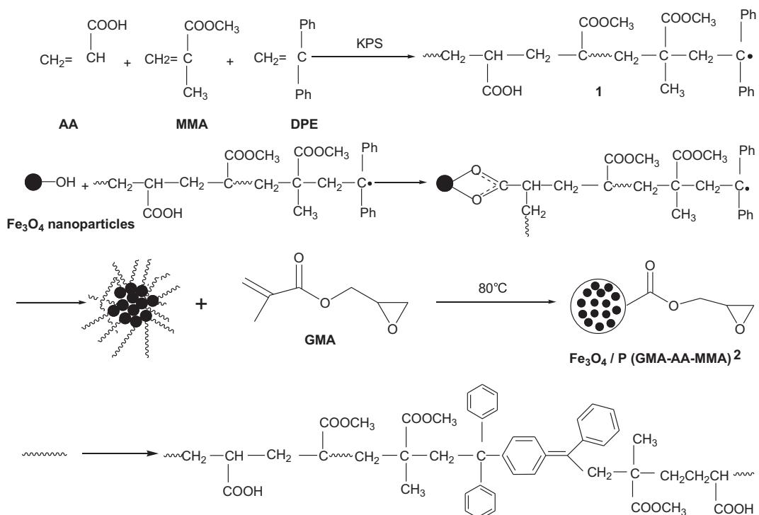
Scheme 1. Synthesis of  $\text{Fe}_3\text{O}_4/\text{P}(\text{GMA-AA-MMA})$ .
