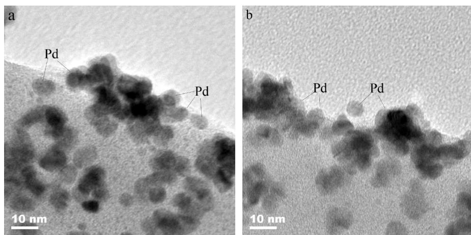
**Fig. 4.** HRTEM micrographs of  $\text{Fe}_3\text{O}_4/\text{P}(\text{GMA-AA-MMA})-\text{Pd}$  before (a) and after (b) Suzuki reaction.
