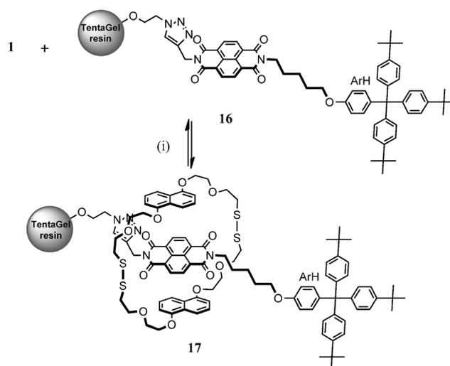
**Scheme 7.** Dynamic synthesis of disulfide-linked naphthalene diimide [2]rotaxane **17**. Reagents and conditions: (i) 1 equiv DBU,  $\text{CHCl}_3$ , air, RT, 14 days.
