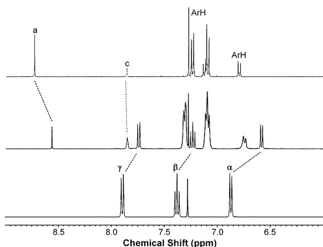
**Figure 6.** Aromatic region of the  $^1\text{H}$  NMR spectra of naphthalene diimide dumbbell **5** (top), [2]rotaxane **12** (middle), and 1,5-dialkoxynaphthalene **1** (bottom) in  $\text{CDCl}_3$  at 303 K.
