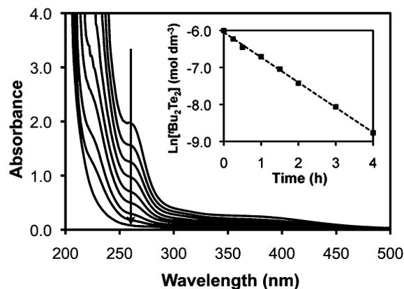
**Fig. 1** Temporal change in the UV-vis spectrum of  ${}^t\text{Bu}_2\text{Te}_2$  during the photolytic decomposition with 254 nm irradiation over 12 h. Apparent first-order reaction kinetics with respect to  ${}^t\text{Bu}_2\text{Te}_2$  (inset).
