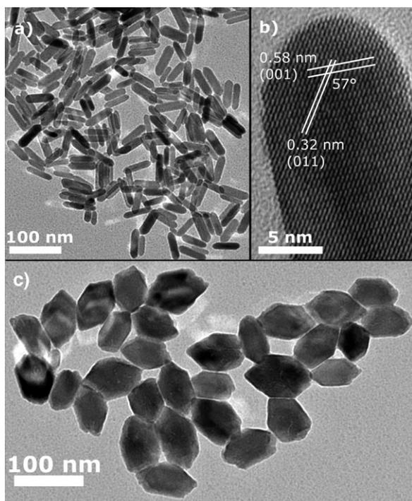
**Fig. 2** TEM images of Te nanorods at (a) low and (b) high resolution. The high resolution image clearly shows the (001) lattice planes lying normal to the nanorod growth direction. (c) TEM image of the ellipsoidal Te nanocrystals formed without the addition of dodecanethiol.
