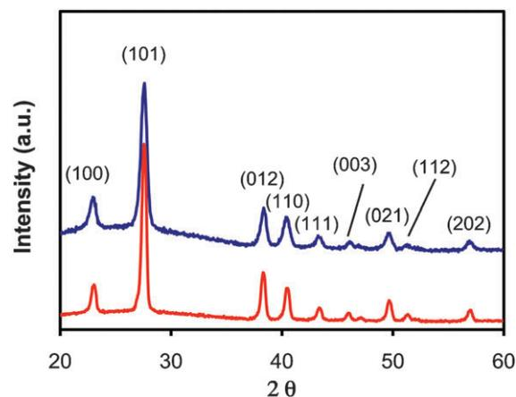
**Fig. 3** XRD pattern of the nanorods (blue) and ellipsoidal nanocrystals (red) indexed to the trigonal phase of tellurium.
