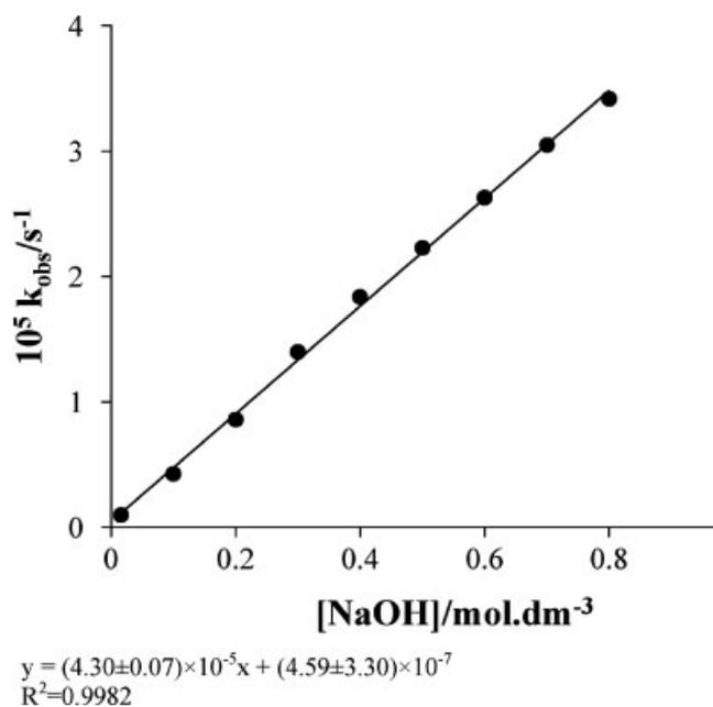
**Figure 5.** Effect of NaOH concentration on the rate of reaction for compound **2** (including the point obtained by graphical extrapolation for hydrolysis in piperidine buffer pH 12.2) in 15% 1,4-dioxane/water (v/v), with  $\mu = 1.0 \text{ mol} \cdot \text{dm}^{-3}$  ( $\text{NaClO}_4$ ), at a temperature of  $27.0^\circ\text{C}$
