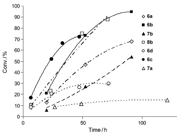
**Figure 3.** Time-conversion curves obtained from ROPs of LA in CH<sub>2</sub>Cl<sub>2</sub> at RT ([10a]/[catalyst]/[BnOH]/[S] = 200:5:1:1; [10a]<sub>0</sub> = 1 M).
