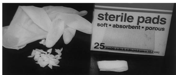
Fig. 1. A photographic depiction of the two fuels: (a) medical examination latex gloves, and (b) sterile cotton pads (gauze), which are abundantly found in “red-bag” medical wastes.
