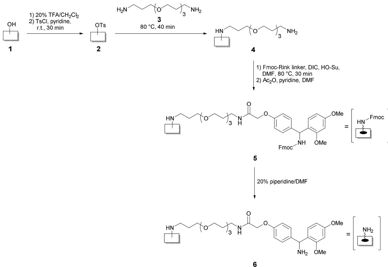
Scheme 1. Preparation of functionalized cellulose support **6** and linker installation.
