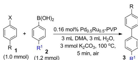
**Scheme 2.**  $\text{Pd}_{0.5}\text{Ru}_{0.5}\text{-PVP}$  NPs-catalyzed SMC reactions of aryl halide (**1**) with arylboronic acid (**2**) under optimized conditions.
