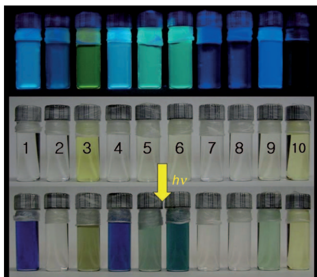
Figure 7. Photographs of compounds 1–10 in toluene showing their colors (middle), fluorescent colors (top), the color change after being irradiated by a UV lamp (365 nm) for \approx 5 min for 1 , 3 , 4 , and 6 and \approx 20 min for all other compounds (bottom).
