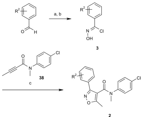
**Scheme 2.** Synthesis of substituted 3-aryl-4-isoxazolecarboxamides. Reagents and conditions: (a) hydroxylamine HCl, NaOAc, EtOH/H<sub>2</sub>O (5:1),  $\mu$ W 150 °C, 1 min; (b) NCS, DMF, 16 h, heat then rt; (c) toluene,  $\mu$ W 160 °C, 10 min.
