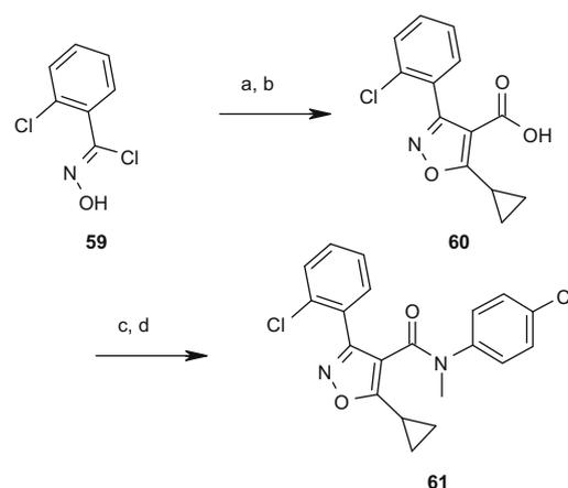
**Scheme 4.** Preparation of 5-cyclopropyl-*N*-methyl-4-isoxazole-carboxamide. Reagents and conditions: (a) ethyl 3-cyclopropyl-3-oxopropanoate, Et<sub>3</sub>N, toluene, rt, 16 h; (b) KOH, EtOH,  $\mu$ W 100 °C, 2 min; (c) oxalyl chloride, cat. DMF; (d) *N*-methyl-4-Cl-aniline, Et<sub>3</sub>N,  $\mu$ W 190 °C, 1 min.
