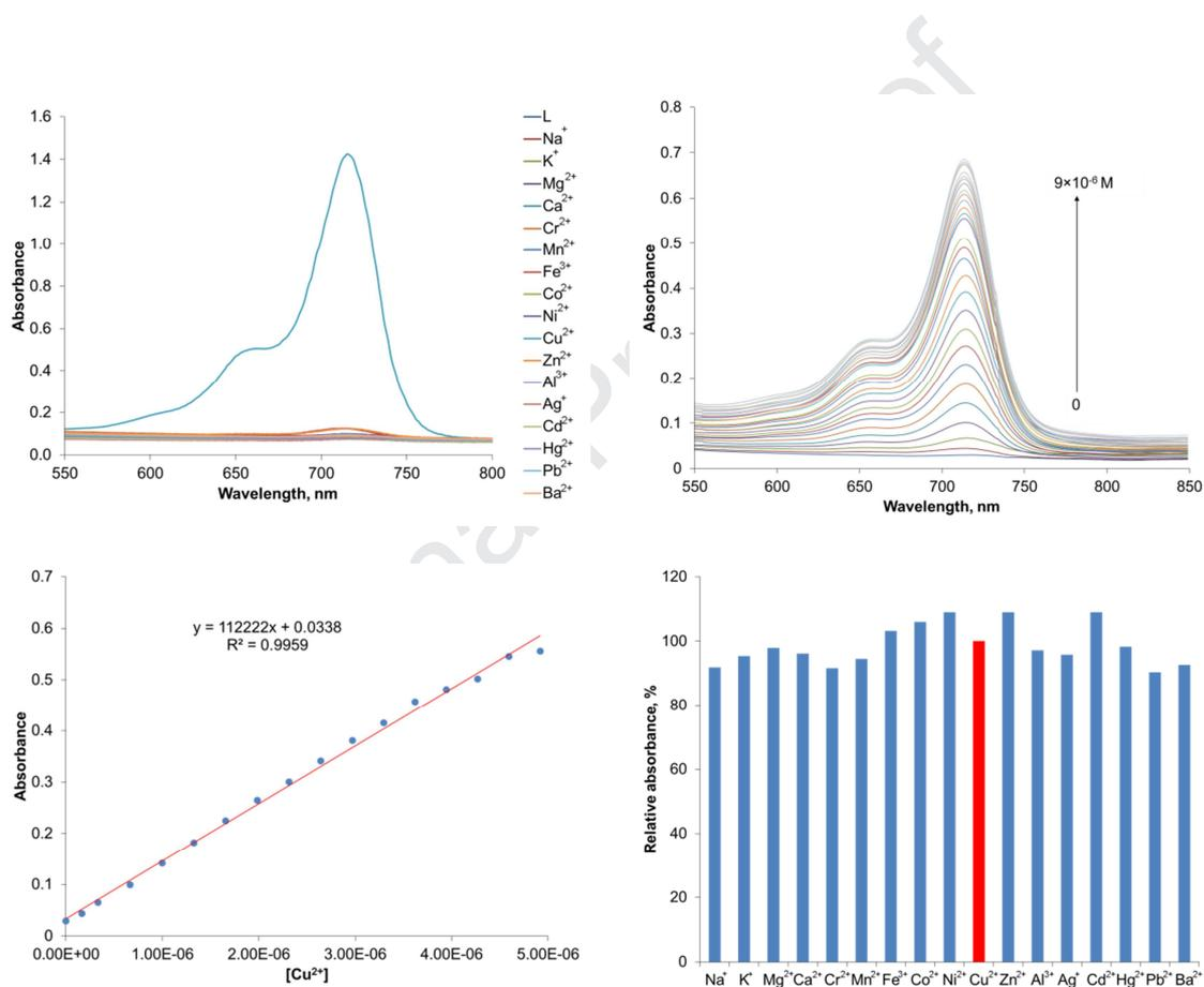
Figure 2. Changes in absorption spectra of sensor (10  $\mu\text{M}$ ) in ethanol/Tris–nitrate buffer (2:1, v/v, pH 7.02) solutions – presence of  $5.0 \times 10^{-5}$  M metal ions (upper left), with various amounts of  $\text{Cu}^{2+}$  ions ( $0$ – $9.0 \times 10^{-6}$  M, upper right), linear working curve derived from titration with  $\text{Cu}^{2+}$  at 710 nm (lower left) and optical response of sensor to  $\text{Cu}^{2+}$  ion among competitive metal ions.
