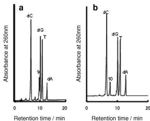
**FIGURE 3** HPLC analysis of the digested **ODN1** (a) and **ODN2** (b) by snake venom phosphodiesterase and alkaline phosphatase. HPLC condition: column, Wakosil 5C18 (4 mm i.d. × 250 mm); eluent, A, 50 mM TEAA (pH 7.2), B, 50 mM TEAA in 70% CH<sub>3</sub>CN; gradient, 3–53%B in 35 minutes; flow rate, 1.0 mL/min.
