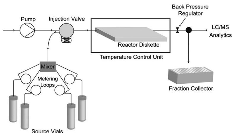
**Figure 1.** Conjure flow reactor, schematic drawing.
