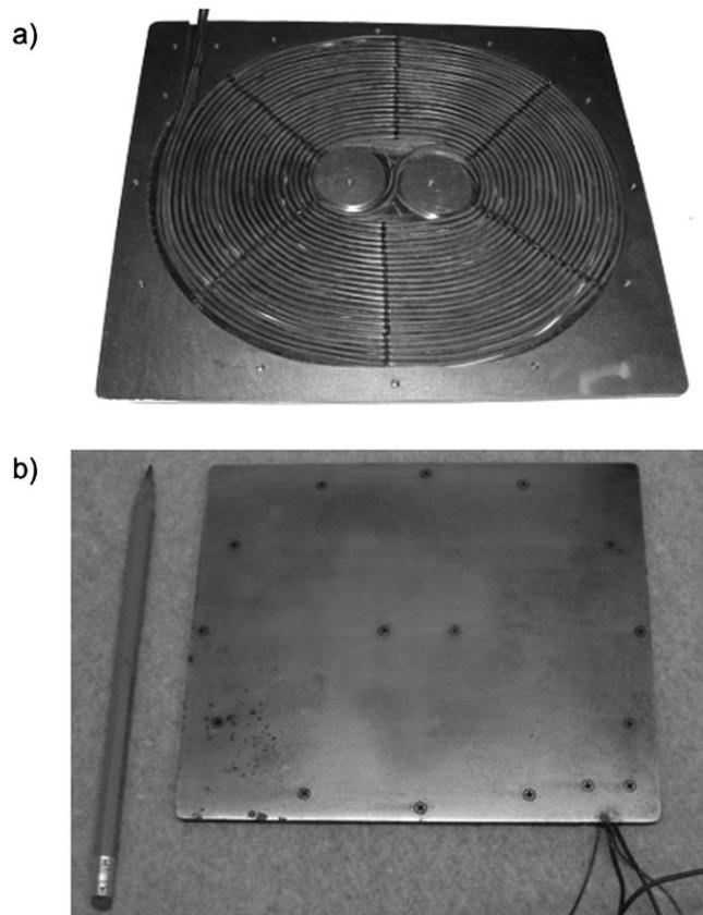
**Figure 2.** a) A reactor diskette with the top copper plate removed, exposing the copper tubing within (0.75 mm i.d.). b) An assembled reactor diskette for the flow reactor (145 mm  $\times$  165 mm  $\times$  5 mm).
