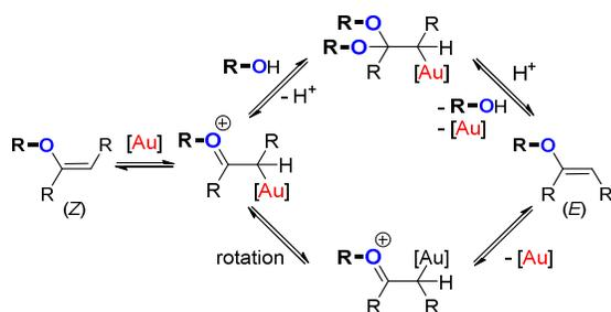
To shed light on the isomerization process, the direct isomerization reactions of pure vinyl ethers (**Z-4a** and **Z-6d**) catalyzed by digold catalyst **1c** and monogold catalyst **1e** were surveyed (Table 4). As expected from the high stereoselectivity obtained in reactions (Schemes 2-3) involving 1-phenylethanol (**3a**), isomerization of vinyl ether (**Z-4a**) was found to be slow (Table 4, entry 1).
