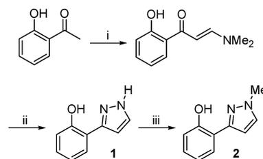
**Scheme 1** (i) DMFDMA, microwave irradiation, 650 W, 5 min.; (ii)  $N_2H_4 \cdot H_2O$ , EtOH, reflux, 4 h; (iii) NaH, MeI, THF, RT, 16 h.
