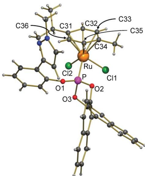
**Fig. 3** Solid state structure of **6**; the disordered solvent molecules are omitted for clarity. Characteristic bond lengths [Å], angles [deg] and dihedral angles [deg]: Ru–Cl1 2.3876(14), Ru–Cl2 2.4211(14), Ru–P 2.2351(13), Ru–C31 2.246(6), Ru–C32 2.267(6), Ru–C33 2.235(6), Ru–C34 2.192(6), Ru–C35 2.156(6), Ru–C36 2.208(6), C11–Ru–Cl2 89.03(5), Cl1–Ru–P 85.50(5), Cl2–Ru–P 88.10(5), C11–C12–C22–C21 –55.2(6), C2–C3–C5–C6 –49.0(8).
