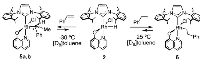
**Scheme 2.** Insertion of styrene into the rhodium–hydride bond monitored by variable-temperature NMR spectroscopy.
