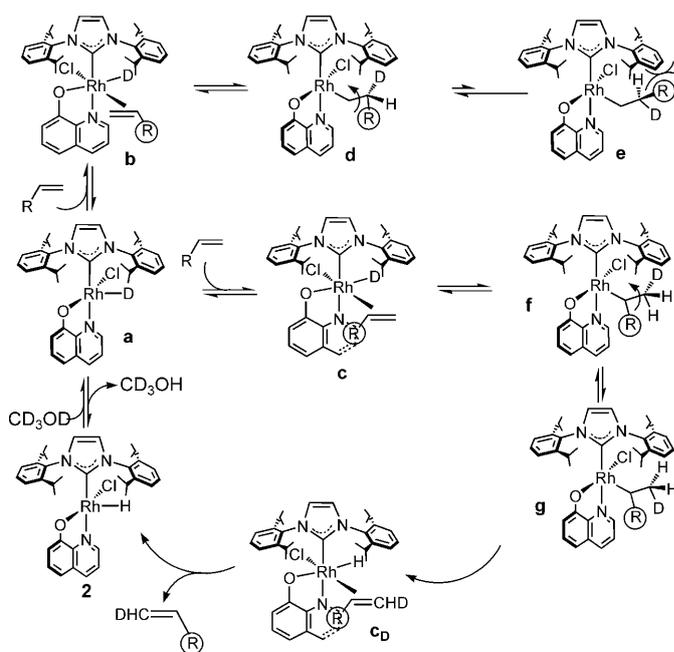
**Scheme 3.** IPr-controlled steric induction for selective H/D exchange.
