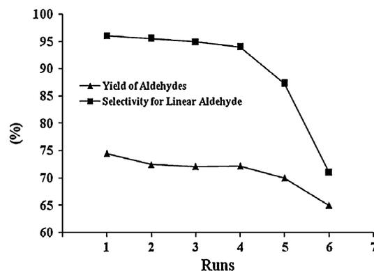
**Fig. 2** Recycle of Rh/1 catalytic system for 2-butene isomerization–hydroformylation [Rh] =  $5.0 \times 10^{-2}$  mmol, 2-butene (20 g), S/C = 7,143, L/[Rh] ratio = 5, *T* = 120 °C, *t* = 2 h, toluene (20 mL) as solvent, heptanes as internal standard, maintain constant pressure (2.5 MPa) during the reaction
