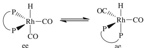
**Scheme 1** Equilibrium of ee–ae configurations in rhodium trigonal bipyramidal complexes
