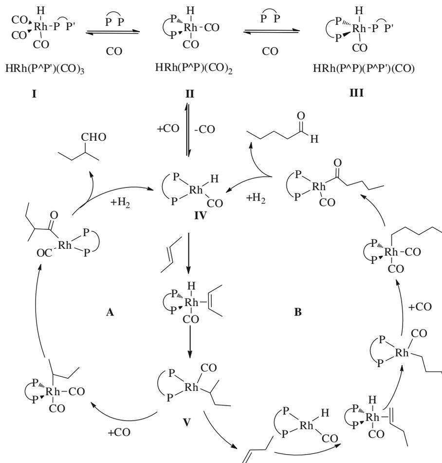
(A) hydroformylation of internal olefin, (B) isomerization–hydroformylation of internal olefin
