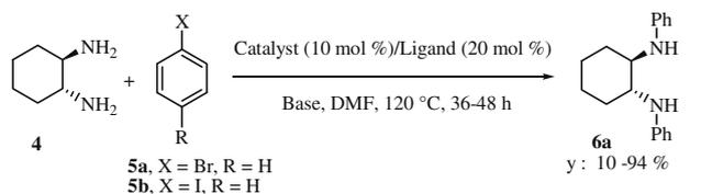
Scheme 1. Coupling of *trans*-(1*R*,2*R*)-diaminocyclohexane (**4**) and halobenzene in the presence of copper(I) catalyst.
