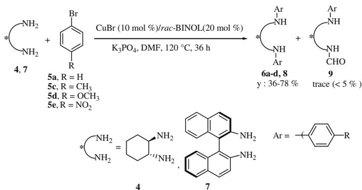
**Scheme 2.** Synthesis of *N,N'*-diaryl chiral  $C_2$ -symmetric diamines.
