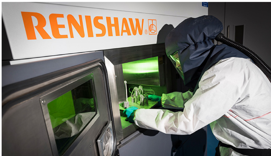
BAE owns several Renishaw 3D printers at its new product development and process development center (NPPDC).
