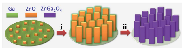
Fig. 7 Schematic illustration for the preparation of \text{ZnGa}_2\text{O}_4 nanorods: (i) solution-liquid-solid (SLS) growth for Ga-doped ZnO nanorods and (ii) topological-morphology-conversion (TMC) process for \text{ZnGa}_2\text{O}_4 nanorods.
