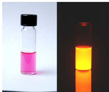
Figure 3. Solutions of 3 in methanol under room light (left) and long wavelength fluorescent light (right).
